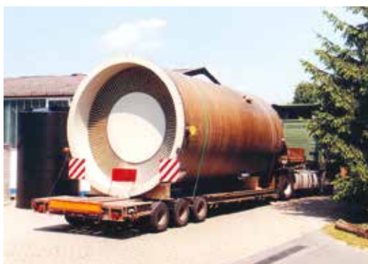
Körting droplet separator during transportation and installed on the chimney of a plant.
